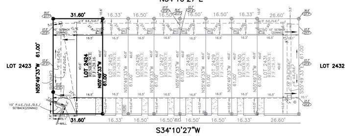
TOP OF CURB ELEV.=26.47 8713 DAYBREAK STREET F €=26.56' (72' PVT. ACCESS/D.D.E./P.U.E.) SEE ARCHITECTURAL PLANS FOR FOUNDATION DESIGN PROPOSED FINISHED FLOOR ELEVATION PER THIS PLAN DRAINAGE SLOPE VARIES EXISTING GROUND FINAL SURVEY DRAINAGE SECTION A-A SCALE: 1'' = 30'
