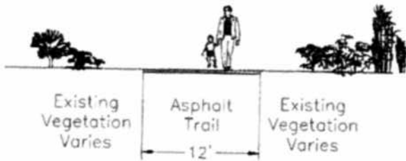
IMPROVED TRAIL 12' Asphalt Pavement Within FPL Easement Area
