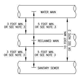
CONDITION "A": WATER MAIN CROSSING OVER RECLAIMED MAIN/SEWER MAIN
